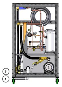
Cooling water "To Process" and "From Process" connections are made at the female NPT couplings provided outside the unit.
